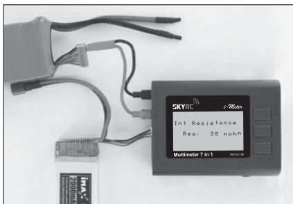
Connection Diagram for Measurement of Battery Internal Resistance
