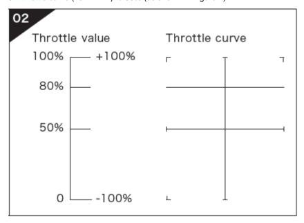
So next time, when you fly your helicopter, let it take off in the "Normal" mode first and then switch to the "IDLE1" mode directly, then your helicopter can starts the 3D flight with 80% throttle amount (that's the standardized speed of 2700 RPM).
