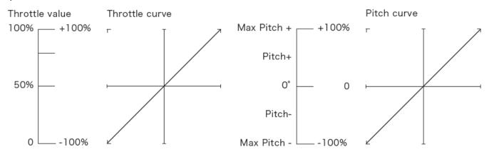
**Attention:** Please ensure the main blade pitch is 0° and the throttle amount is above 40% (we recommend using 50%) when standardizing the speed.
