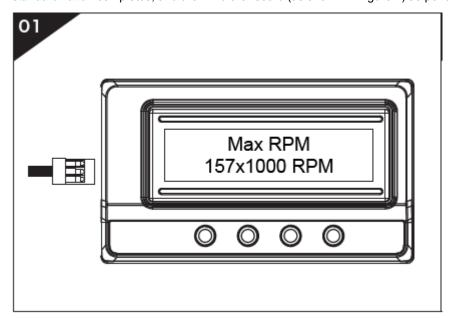
The value shown in the image is just an example, pleas take the value actually displayed on your LCD program box as standard. This value is the max. electrical RPM the motor can reach at the 100% throttle.
