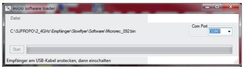
Connect channel 5 of the receiver to the USB update cable and then turn it on. The LED expires and the progress-bar shows you the progress of the firmware update. The update is complete when the bar reaches the right end and the red LED on the receiver starts flashing. Because the receiver settings remain after the update, the receiver can be used immediately.
