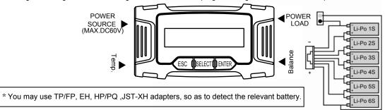
It shows the type of battery and number of cell-count at upper right, and output voltage. At lower line, it displays the residual capacity at percentage and visual graph.
