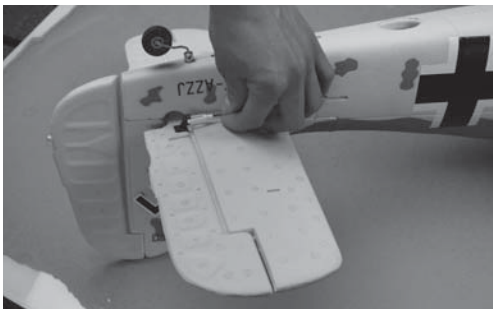
11 Install elevator push rod as shown.
