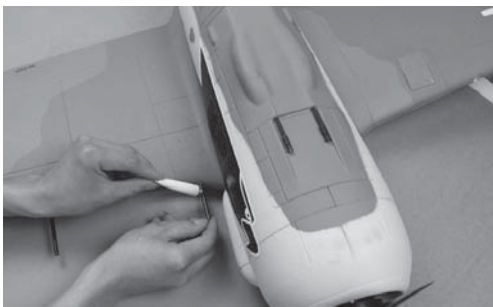
15 Glue the short plastic scale gun on the wing.
