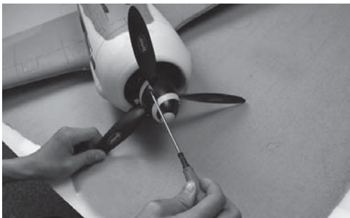
13 Install spinner with PA2.5x8mm screws.
